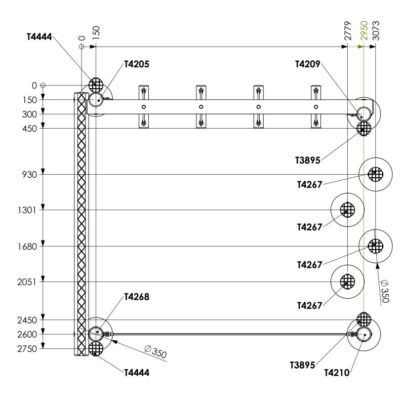
Dig groundworks 600mm deep on the stepping logs and 763mm deep for the 4 main timber legs
