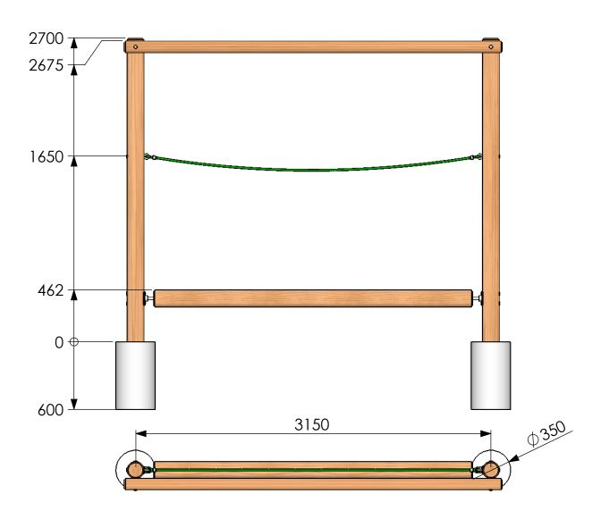
No safety surface required as critical fall height is less than 600mm. However we suggest allowing an appropriate free space around the item in compliance with BS EN1176.
