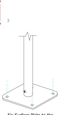
Fix Surface Plate to the ground surface Ground **Anchors Not provided** cover fixings with caps provided
