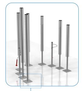
**1**. Attach Surface Fixing plates to each of the 9 legs(1.2)
