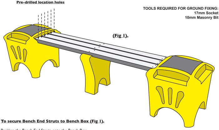
Position the Bench End Struts onto the Bench Box.
