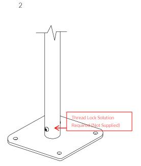
Fix instrument to Surface fix plate using M10 bolt and Barrel Nut and use **thread locking solution** to prevent fixings working loose.
