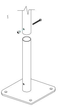
Locate the Surface fix Plate into the leg of the instrument.
