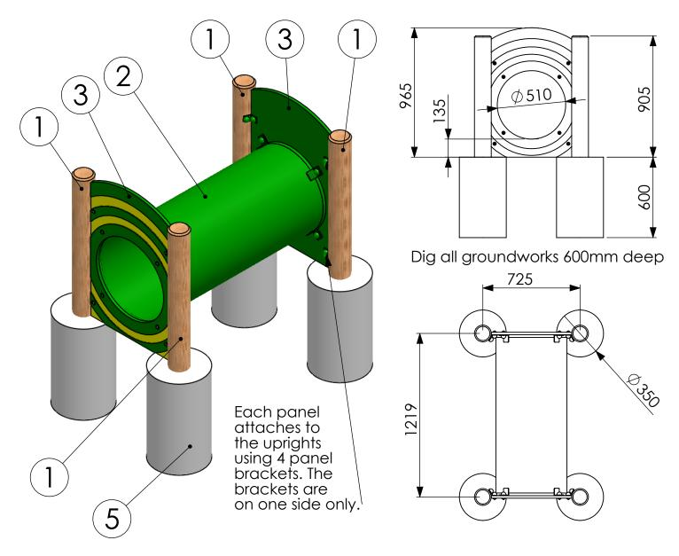
No safety surface required as critical fall height is less than 600mm. However we suggest allowing an appropriate free space around the item in compliance with BS EN1176.
