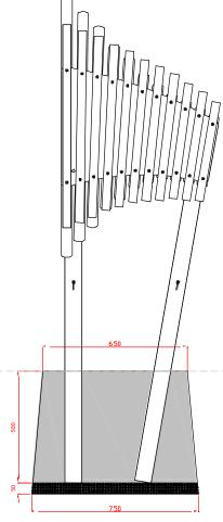
Fill hole with fast drying concrete to manufacturers specifications. If posts protrude above instrument they can be cut down
