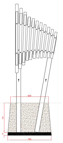
Compact base of hole with 50mm of aggregate. Lower ground Fix posts attached to instrument into hole (check instrument straight and level, and at correct height before filling with concrete)
