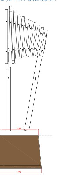
Excavate a hole with a 250x650mm tapering down to 350x750mm diameter and 550mm depth
