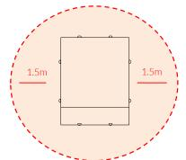
Install Instrument with 1.5m free space (from widest point) around it.
