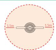
Install Instrument with 1m free space (from widest point) around it.
